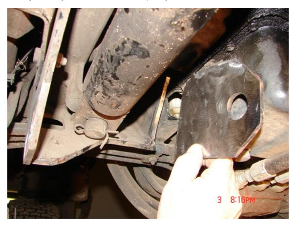
After tacking the piece in place, temp welded a support bar across to keep the piece from warping while doing the hard weld. The mig was a lifesaver as it is real tight in there.
