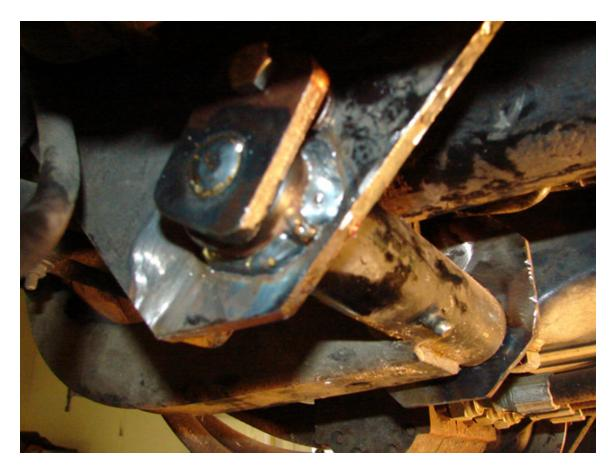
Now everything is in place, new rod and lift arm inserted and bolted in place, temp support cut out.
