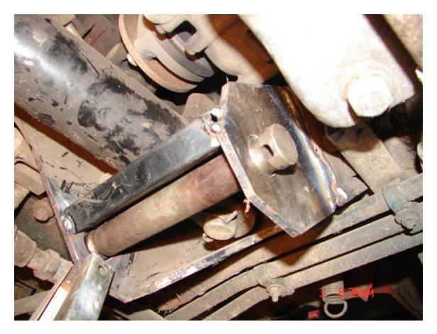
To aid in further support for the pivot rod, on each side of the framing I welded on a bearing lock collar.
