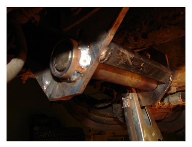
To keep the rod from spinning, took a piece of flat stock and welded it to the rod and drilled another hole for a bolt to lock it into the frame in the existing hole in the frame. Much greater strength than the original design.
